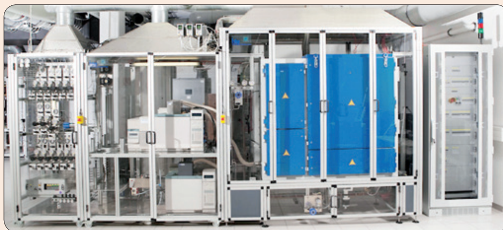
Fig. 2: 16-fold high throughput reactor system for high pressure operation. The unit is designed to perform reactions relevant for refinery catalysis and fuels upgrading like hydrodesulfurization, hydrodenitrogenation or hydrodeoxygenation (source: hte GmbH).
